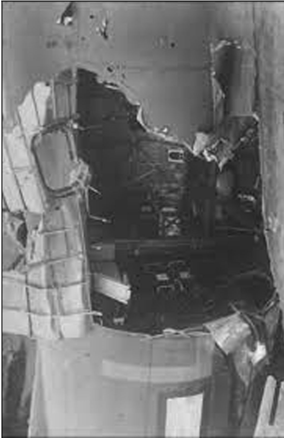
The gapping 7' x 12' hole in the side of the fuselage of "Miss Irish."
