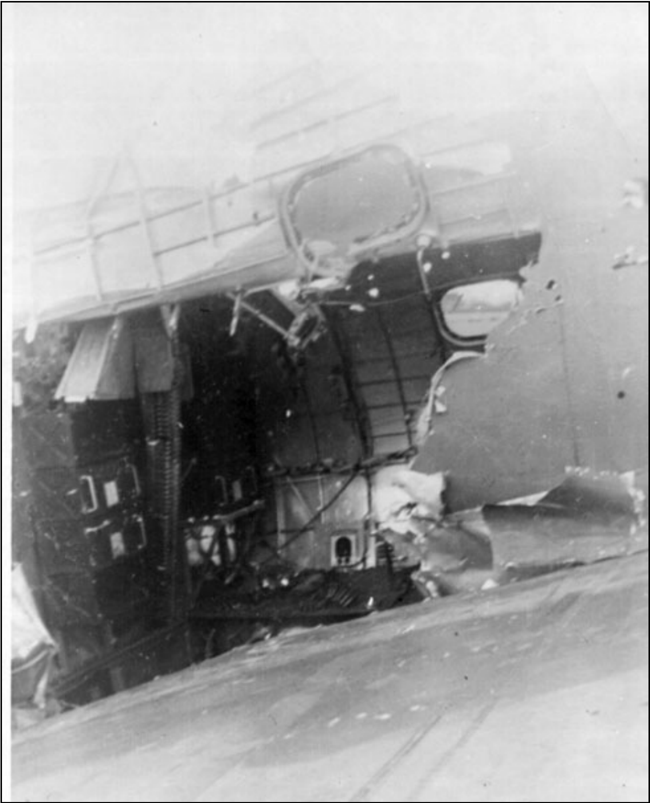
The aft bulkhead can be seen in the rear portion of the Radio Operator's compartment. The bulkhead was the only thing that held the stricken bomber from breaking in half.
