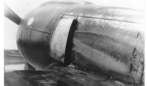
Above is the side exhaust of the La-5F, and below the side exhaust of the La-5FN. The small bump can be produced from scrap plastic, and in 1/72 scale does not really have to be hollowed out.
