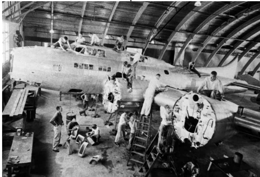
B-17 in Lysdale Flying Service hangar undergoing refurbishment
